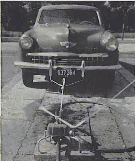
SPRINKLER TOWS CAR along the hose, slowly but surely, sprinkling as it goes. Car weighs 2,700 pounds.
