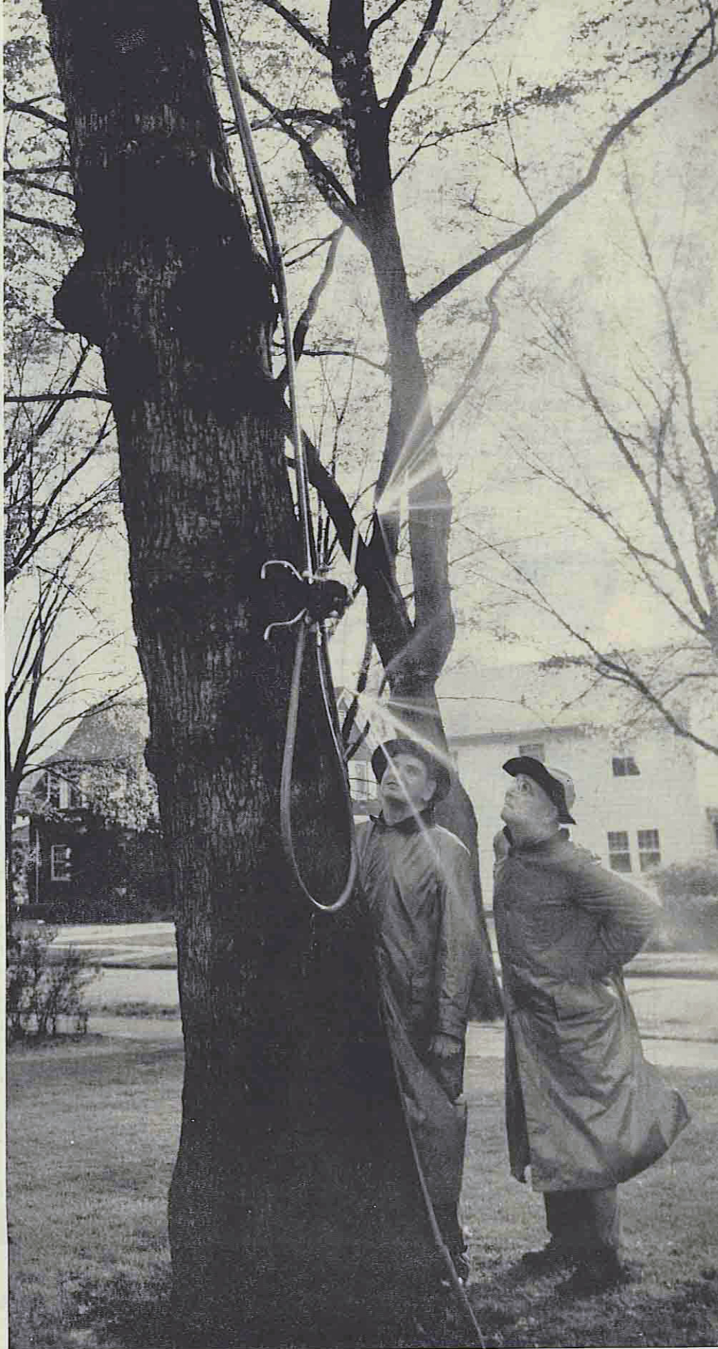
SPRINKLER CLIMBS TREE by pulling itself up its own hose which is fastened to a limb. South Bend, Ind.
